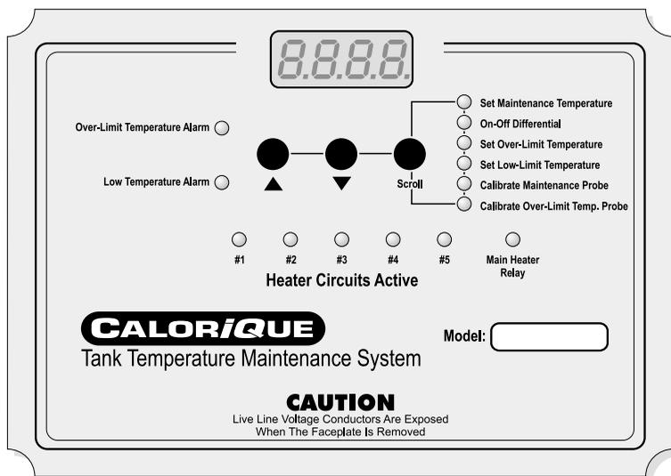
The over-limit and low-limit temperatures are used in conjunction with the on-board indicator lights and/or remote alarms to indicate a fault situation. If the over-limit temperature is reached, power to all elements will be shut off.
